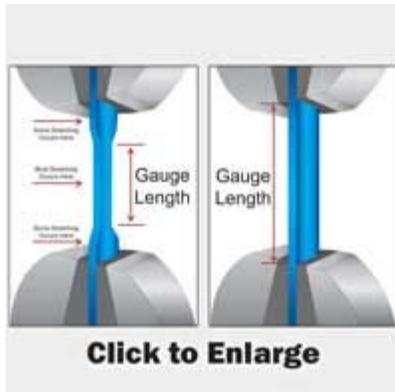
For specimens that have the same cross-sectional area from end to end (tubes, rods, rectangles and fibers), the gauge length is determined by simply measuring the distance between the grip faces (refer to image).
