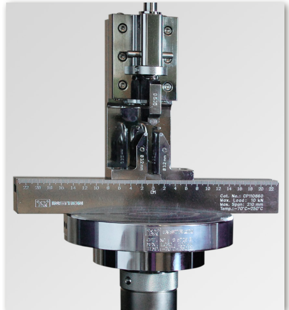
ILSS Testing to ASTM D2344 with CP107574 Anvils on Base Fixture
